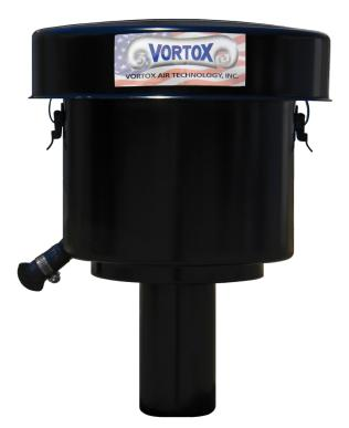
The AP120J4 is a multi-stage, pressure only air cleaner primarily used in conjunction with Gardner Denver/Drum 450 blower applications, both truck mounted and stationary. The AP120J4 air cleaner has an integrated inlet design that requires no additional accessories. The 4" OD outlet tube is well suited for applications up to 400 CFM.
