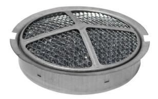
Before replacing the cup, remove the prefilter by pressing upward, turning to the left until the locking tans line up with the vertical slots, and then pull downward. The prefilter should be washed clean in detergent and hot water each time the cleaner is serviced since it is designed to stop lint, chaff, and fibrous material from entering the main filter element. Replace the prefilter and install the cup making sure the disc and the proper amount of oil are in the cup.
