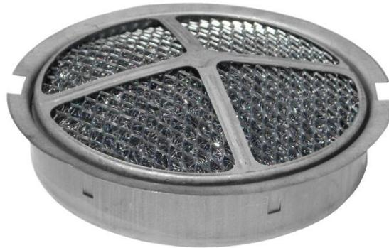
Before replacing the cup, remove the prefilter by pressing upward, turning to the left until the locking tabs line up with the vertical slots, and then pull downward. The prefilter should be washed clean in detergent and hot water each time the cleaner is serviced since it is designed to stop lint, chaff, and fibrous material from entering the main filter element. Replace the prefilter and install the cup making sure the disc and the proper amount of oil are in the cup.
